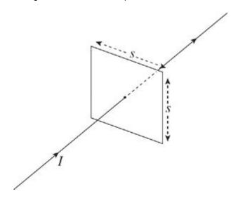
If the current in the wire is *I*, determine the current induced in the square loop.
