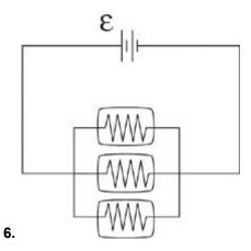
Three identical light bulbs are connected to a source of emf, as shown in the diagram above. What will happen if the middle bulb burns out?
