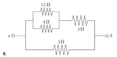
Determine the equivalent resistance between points *a* and *b*.
