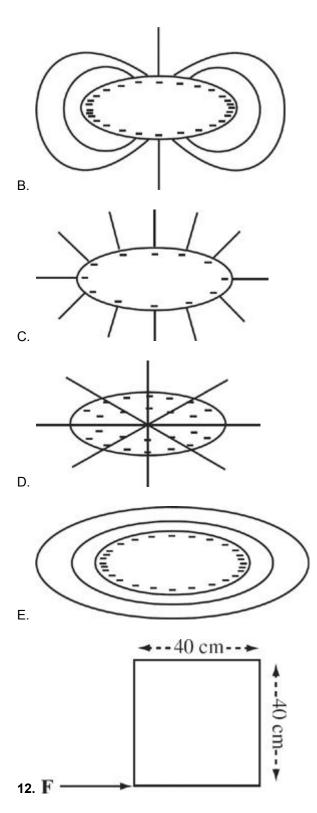
The figure above shows a square metal plate of side length 40 cm and uniform density, lying flat on a table. A force **F** of magnitude 10 N is applied at one of the corners, parallel to one of the sides, as shown. What's the torque produced by **F** relative to the center of the square?
