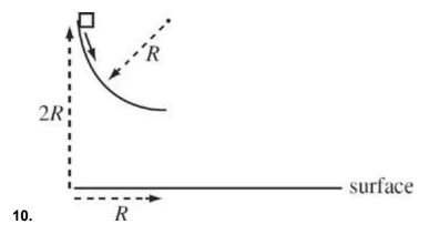
A small box slides down a frictionless track in the shape of a quarter-circle of radius *R*. The box starts from rest at the top of the track, a height equal to 2*R* above a horizontal surface. At the moment the box leaves the bottom of the track, a ball of the same mass as the box is dropped from the same height at the bottom of the track.
