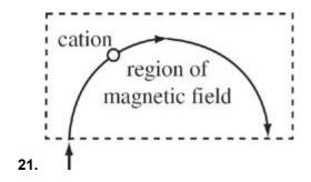
The figure above shows a cation (a positive ion—that is, an atom that has lost one or more electrons) entering a mass spectrometer, which contains a region with a uniform magnetic field, **B**. Once in the magnetic field, the cation moves in a semicircular path in the direction indicated. What is the direction of **B**?
