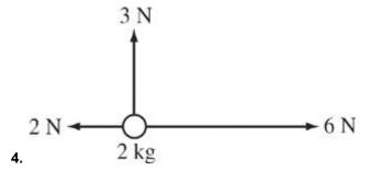
The figure above shows the forces acting on an object of mass 2 kg. What is the object's acceleration?
