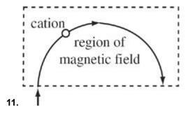
The figure above shows a cation (a positive ion—that is, an atom that has lost one or more electrons) entering a mass spectrometer, which contains a region with a uniform magnetic field, **B**. Once in the magnetic field, the cation moves in a semicircular path in the direction indicated. What is the direction of **B**?
