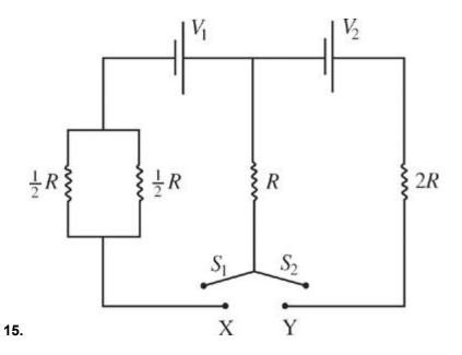
The circuit shown contains two switches:  $S_1$ , which can connect to point X, and  $S_2$ , which can connect to point Y.
