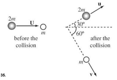
An object of mass 2m moving with velocity **U** strikes an object of mass m initially at rest. After the collision, the objects move away with velocities **u** and **v**, as shown.
