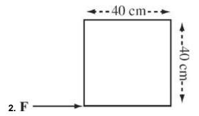
The figure above shows a square metal plate of side length 40 cm and uniform density, lying flat on a table. A force **F** of magnitude 10 N is applied at one of the corners, parallel to one of the sides, as shown. What's the torque produced by **F** relative to the center of the square?
