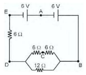
Through which point does half the total current pass?
