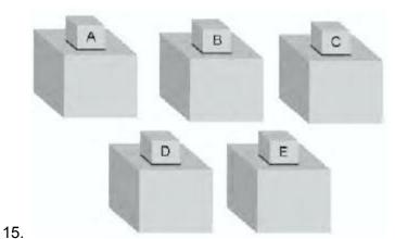
Five blocks having equal mass but made of different substances, as shown above, are heated to 100°C and placed on separate 10 kg blocks of ice that are at a temperature of 0°C. Which substance melts the greatest amount of ice?
