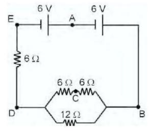
At which point is all the voltage in the circuit dropped to zero?
