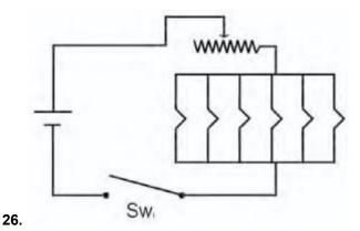
The diagram above shows a battery and a variable resistor set at its midpoint resistance in series with a parallel light circuit. Switch 1 ( $Sw_1$ ) is closed and the light bulbs illuminate. When the variable resistor is moved slightly to the left (L) the bulbs dim a little. When the variable resistor is moved slightly to the right (R) the bulbs brighten slightly. What happens in the circuit when the variable resistor is set all the way to the right?
