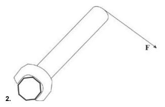
In an effort to tighten a bolt, a force  $\mathbf{F}$  is applied as shown in the figure above. If the distance from the end of the wrench to the center of the bolt is 20 cm and  $\mathbf{F}$  = 20 N, what is the magnitude of the torque produced by  $\mathbf{F}$ ?
