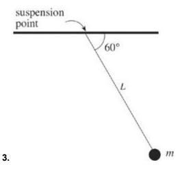
In the figure above, what is the torque about the pendulum's suspension point produced by the weight of the bob, given that the mass is 40 cm below the suspension point, measured vertically, and m = 0.50 kg?
